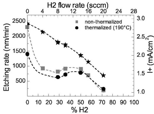
FIG. 7. Positive ion current density (right axis, stars) and etching rate (left axis) of nonthermalized (squares) and thermalized (dots) InP samples as a function of the  $\text{H}_2$  percentage in the  $\text{Cl}_2$ - $\text{H}_2$  gas mixture. The other plasma conditions are  $T=190^\circ\text{C}$ , 0.5 mT, 800 W ICP power,  $-145\text{ V}$  dc bias, and total flow rate of 28 sccm.
