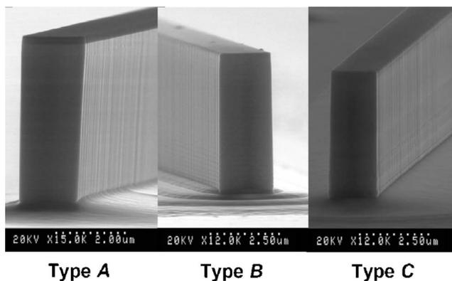
FIG. 11. SEM images of type-A, -B, and -C samples etched with  $T=190^\circ\text{C}$ , 0.5 mT, 800 W ICP power,  $-145\text{ V}$  dc bias, and a total flow rate of 28 sccm. Samples are nonthermalized. The  $\text{H}_2$  percentage is set in the 35%–45% range and the etch depth is  $\sim 5\ \mu\text{m}$ .
