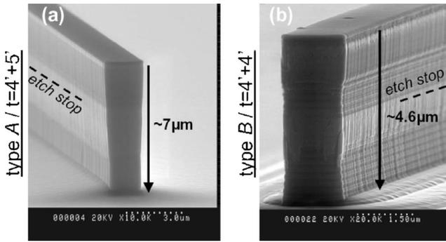
FIG. 10. SEM images of the [(a) and (b)] type-A and (c) type-B samples etched with  $T=190^\circ\text{C}$ , 0.5 mT, 800 W ICP power,  $-145\text{ V}$  dc bias, and  $\text{Cl}_2/\text{H}_2=20/8$  sccm in a two-step etch. The samples are nonthermalized.
