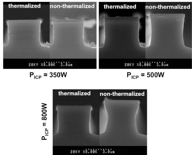
FIG. 6. Cross-section SEM images of thermalized (left) and nonthermalized (right) InP samples etched for  $T=190\text{ }^{\circ}\text{C}$ , 1 mT, -145 V dc bias,  $\text{Cl}_2/\text{H}_2=10/4$  sccm, and for ICP powers of 350, 500, and 800 W.
