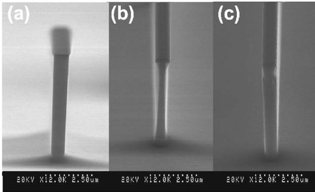
FIG. 4. SEM images of nonthermalized InP samples etched for 5 min with  $T=190\text{ }^{\circ}\text{C}$ , 0.5 mT, 800 W ICP power, -145 V dc bias, and  $\text{Cl}_2/\text{H}_2=18/10$  sccm. (a) Silicon carrier. (b) Aluminum carrier. (c) Aluminum carrier with silicon pieces.
