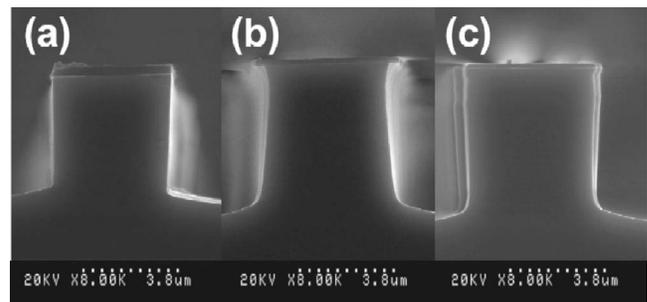
FIG. 3. Cross-section SEM images of nonthermalized InP samples etched for 7 min with  $T=190$  °C, 0.5 mT, 800 W ICP power,  $-145$  V dc bias, and  $\text{Cl}_2/\text{H}_2=20/8$  sccm. (a) Silicon carrier. (b) Aluminum carrier. (c) Aluminum carrier with silicon pieces.
