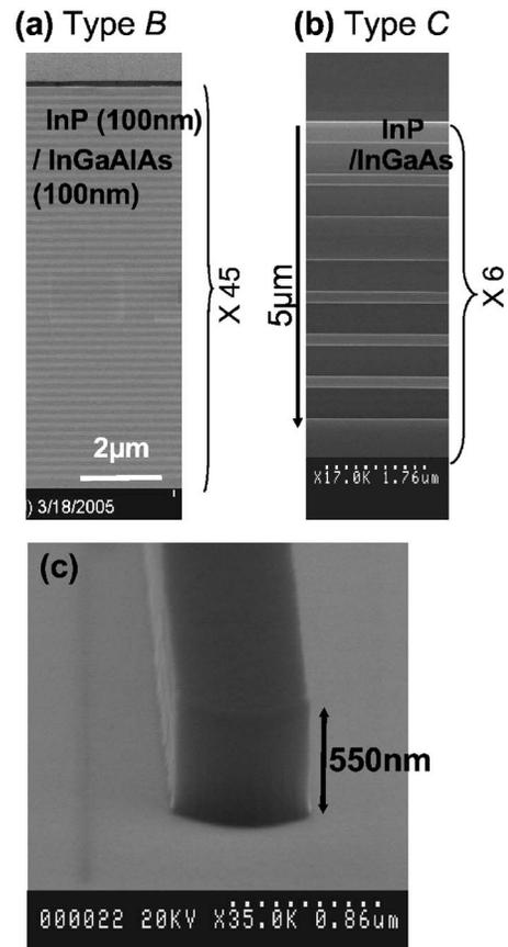
Fig. 1. Cross-section SEM images of the (a) type-B and (b) type-C structures. (c) SEM image of the dielectric mask.
