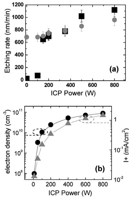
FIG. 5. (a) InP etching rate measured as a function of ICP power for thermalized (dots) and nonthermalized (squares) samples, with  $T=190\text{ }^{\circ}\text{C}$ , 1 mT, 500 W ICP power, -145 V dc bias, and  $\text{Cl}_2/\text{H}_2=10/4$  sccm. (b) Electron density (dots, left axis) and positive ion current density (triangles, right axis) measured as a function of ICP power under the same plasma conditions.
