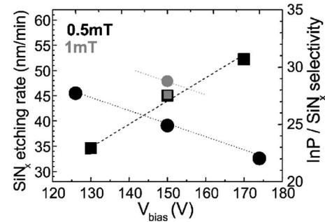
FIG. 12. Etching rate of the rf-PECVD  $\text{SiN}_x$  material (dots) and selectivity of  $\text{SiN}_x$  mask over InP (squares) measured for 800 W ICP power,  $\text{Cl}_2/\text{H}_2=20/8$  sccm, and working pressures  $P=0.5\text{ mT}$  (black color) and  $P=1\text{ mT}$  (gray color). The dc bias is varied between  $-130$  and  $-170\text{ V}$  for  $P=0.5\text{ mT}$ . The electrode temperature was set to  $150^\circ\text{C}$  and the samples are nonthermalized.
