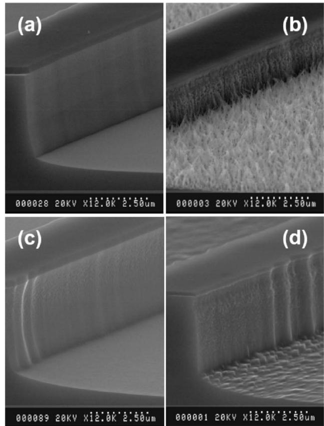
FIG. 2. SEM images of [(a) and (b)] thermalized and [(c) and (d)] nonthermalized InP samples etched for 5 min with  $T=190$  °C, 1 mT, 500 W ICP power,  $-145$  V dc bias, and  $\text{Cl}_2/\text{H}_2=10/4$  sccm. [(a) and (c)] Silicon carrier. [(b) and (d)] Aluminum carrier.
