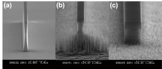
FIG. 8. SEM images of the InP samples etched for 5 min in the conditions of Fig. 7 for a  $\text{H}_2$  percentage of (a) 0%, (b) 57%, and (c) 70%. The samples are nonthermalized.
