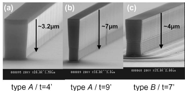
FIG. 9. SEM images of the [(a) and (b)] type-A and (c) type-B samples etched with  $T=190^\circ\text{C}$ , 0.5 mT, 800 W ICP power,  $-145\text{ V}$  dc bias, and  $\text{Cl}_2/\text{H}_2=20/8\text{ sccm}$ . The etching time is (a) 4 min., (b) 9 min., and (c) 7 min.. The samples are nonthermalized.
